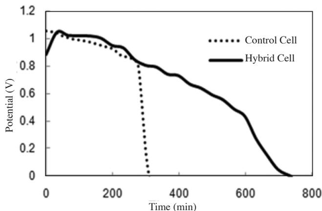
FIGURE 4. A comparison between discharge profiles of an enzymatic zinc-air cell and a negative control (without laccase) to substantiate the biocatalytic activity of laccase enzyme
