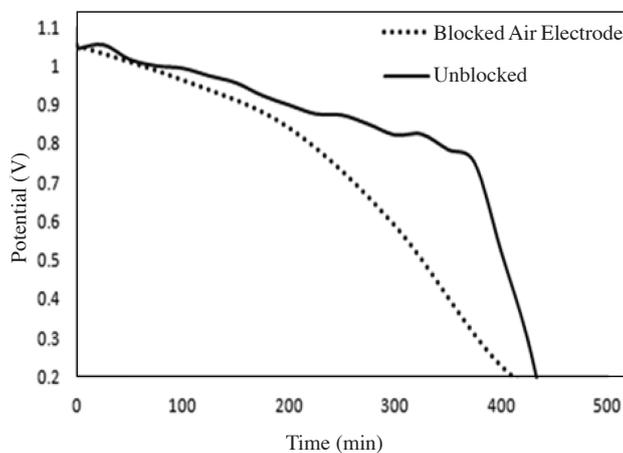
FIGURE 6. Enhanced discharge profile obtained by using the air electrode
