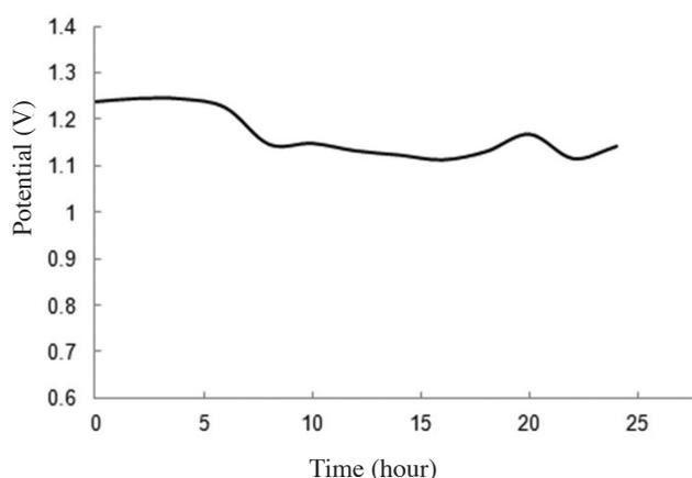
FIGURE 2. OCV of the hybrid cell monitored over 24 h
