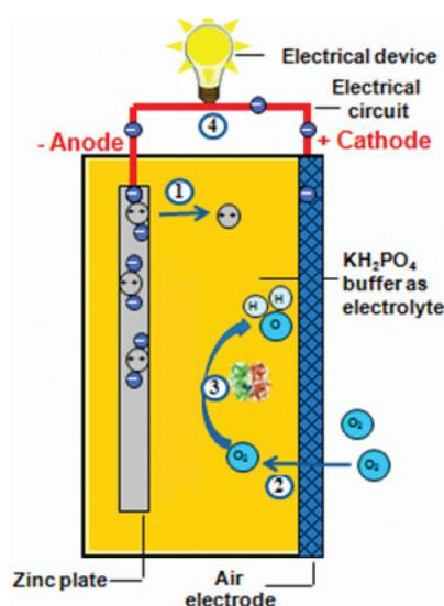
FIGURE 8. Reaction mechanisms of a membraneless, freely suspended laccase of an enzymatic zinc-air biofuel cell
