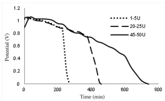
FIGURE 5. Cell discharge capacity with varying biocatalyst concentrations
