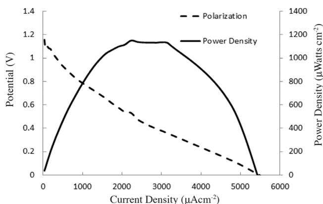
FIGURE 3. Polarization and power density profiles of the hybrid cell
